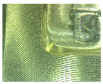
After being stroked a few times on a wet abrasive sheet, I got what I think is a reasonable finish, albeit with a bit of rounding on one edge.
