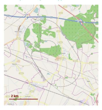
Yes, this is real... About 50km east of Prague there is a 13.25km oval of track which is used for testing, amongst other things, 230km/h tilting trains. Rail operators from all over Europe use it.More at <a href="https://en.wikipedia.org/wiki/Velim\_railway\_test\_circuit">https://en.wikipedia.org/wiki/Velim\_railway\_test\_circuit</a> where you'll find pictures of a Class 92 under test.
