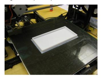
Meanwhile, Peter has been working on detailing. Here is a 3D printed wagon side, complete with strapping.
